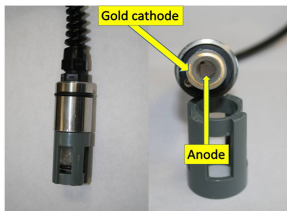
Figure 3. Typical membrane electrode used for measuring dissolved oxygen. A gas-permeable membrane covers the gold cathode and anode. The electrode is attached to an electronic meter that gives direct readings in mg/L or percent saturation.
